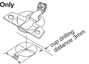
Doors will be drilled 3" from the top and bottom to the center of the 35mm hole. Doors over 40" in length will be drilled for 3 holes. When ordering arch, cathedral or moon styles, please specify right or left hand drilling. Special drilling is available, please send a detailed drawing.
