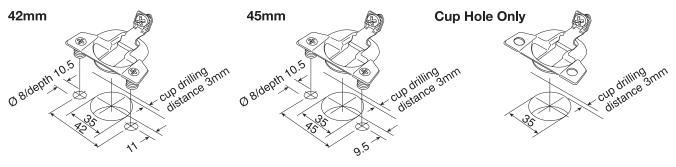
Doors will be drilled 3" from the top and bottom to the center of the 35mm hole. Doors over 40" in length will be drilled for 3 holes. When ordering arch, cathedral or moon styles, please specify right or left hand drilling. Special drilling is available, please send a detailed drawing.
